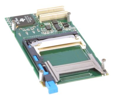
A highly configurable PMC/PCMCIA HBA, the PMC232 integrates PC-Cardbus devices using a PMC form factor with a range of mechanical configurations. As with the PMC230, the PMC232 offers PCMCIA expansion for single board computers or other processor boards supporting PMC connectivity. In addition, card edge PCI systems can be accommodated using GE Fanuc Embedded Systems PMC239 adapter, for rapid prototype and development.
