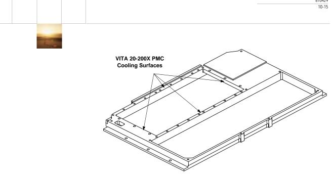
Figure 2: Thermal Frame with VITA 20-200X PMC Cooling Surfaces
