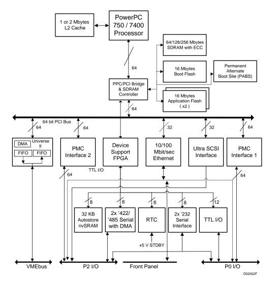
Figure 1: Block Diagram (see Table 3 for alternate I/O Routing)
