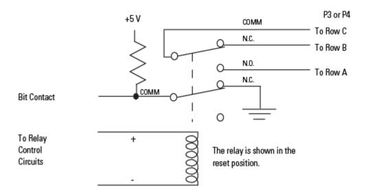
Figure 1. A Typical Relay Circuit
